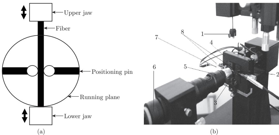
1 — Upper jaw; 2 — Positioning pin; 3 — Lower jaw; 4 — Running plane; 5 — Optical microscope; 6 — CCD camera; 7 — Temperature sensor; 8 — Heater
