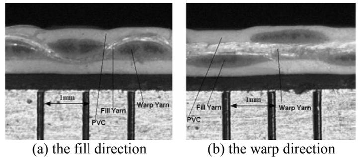
Figure 1 The cross-section of woven PVC-coated membrane material.
