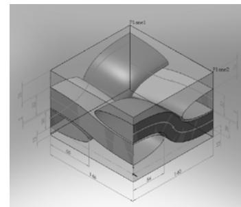
Figure 2 The finite cell of woven membrane material, (unit:  $10^{-2}$ mm).
