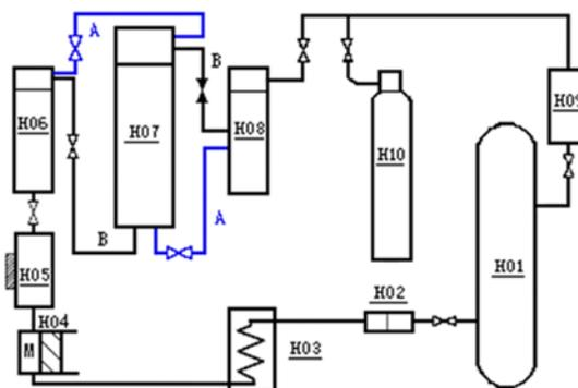
H01-CO<sub>2</sub> Tank H02-Filter H03-Refrigerant container
