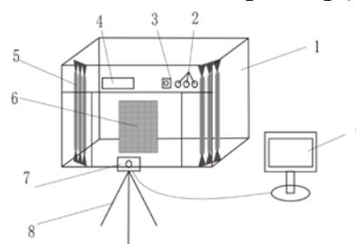
1. Light box; 2. Light box switch knob; 3. Light box switch; 4. Light box panel; 5. Lamp; 6. Vertical wicking setting; 7. CCD camera; 8. Tripod; 9. Computer.
