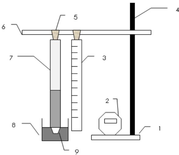
1. Bottom; 2. Stopwatch; 3. Sample; 4. Beam; 5. Sample clip; 6. Vertical bracket; 7. Ruler; 8. Container; 9. Tension clip.
