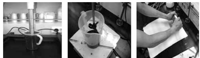
Figure 1 Manufacturing process of PU/MWNT film.
