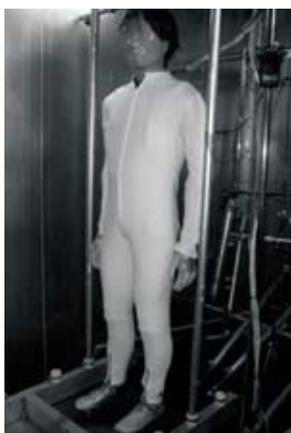
Figure 1 The thermal manikin Tore.
