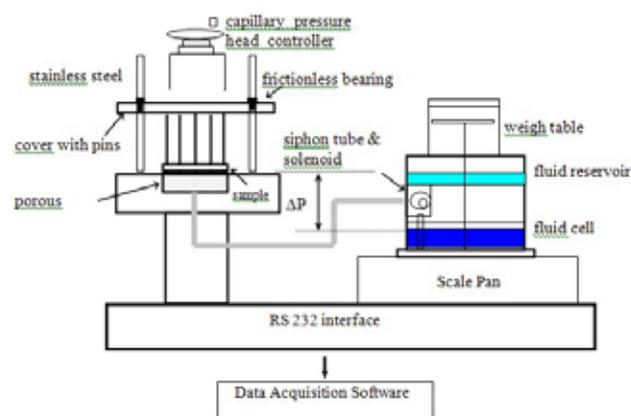
Figure 1 Gravimetric Absorbency Testing System (GATS)
