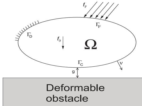
FIGURE 1. Physical setting: an elasto-viscoplastic body in contact with a deformable obstacle.
