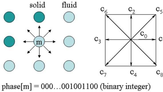
Figure 2: Data structure of the phase information for a two-dimension model.
