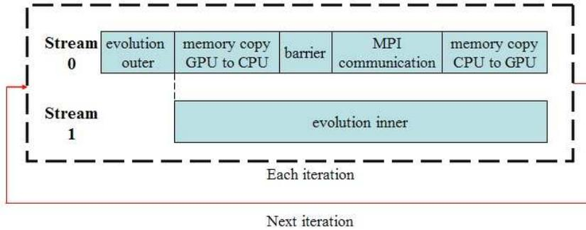
Figure 1: Flow diagram of the overlapped model.
