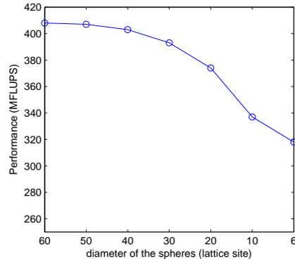
Figure 4: Performance varies with different diameters.
