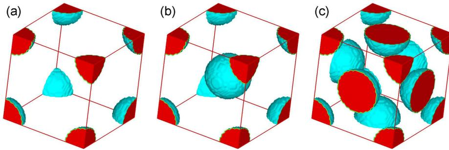
Figure 8: Structure of three cubic arrays of spheres: (a) simple cubic arrays; (b) body-centered cubic arrays; (c) face-centered cubic arrays.
