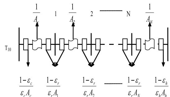
Figure 2 Radiative heat transfer diagram
