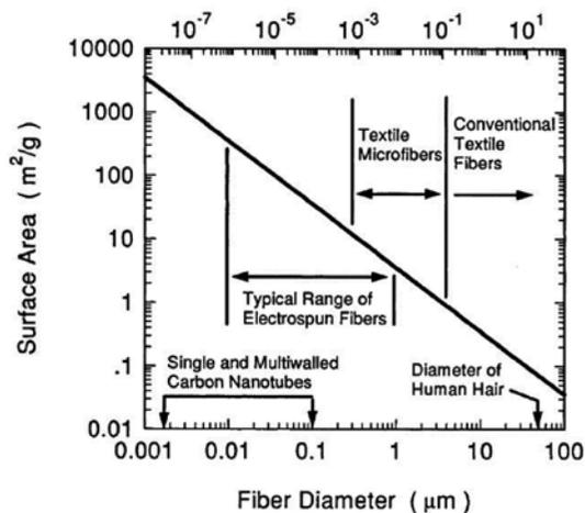
Figure 1 Relationship of fibre diameter to surface area
