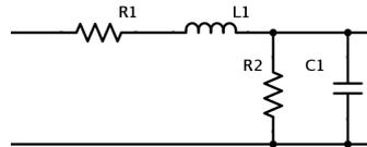
Fig. 1.1. A schematic representation of the elementary components of a transmission line.
